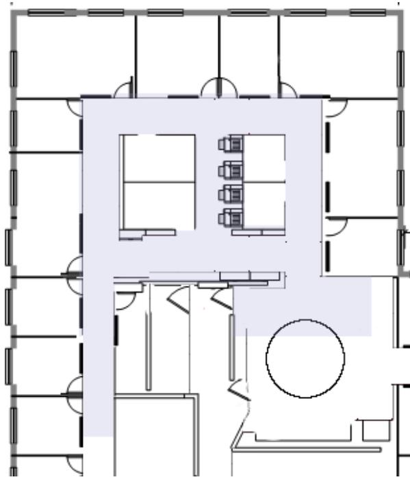
Figure 2: The floor plan of the wing where experiment data was collected. In the very center is a collection of copiers and printers. Surrounding those are a set of cubicles. On the outside are offices. The areas observed by sensors (shaded) are hallways.
