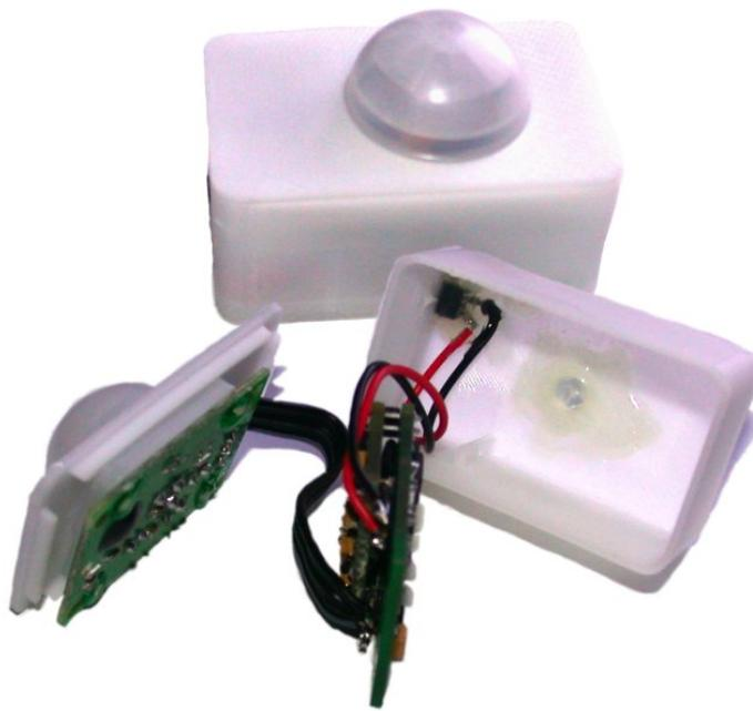
Figure 1: The hardware implementation of the motion detector node.
