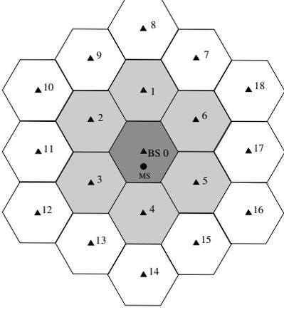
Fig. 1. Hexagonal layout of a 19-cell cellular system.
