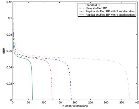
Fig. 1. BER versus number of iterations predicted by density evolution with the standard BP, plain shuffled BP, replica shuffled BP with two and four subdecoders, for decoding (3,6) regular LDPC code at SNR 1.111dB.
