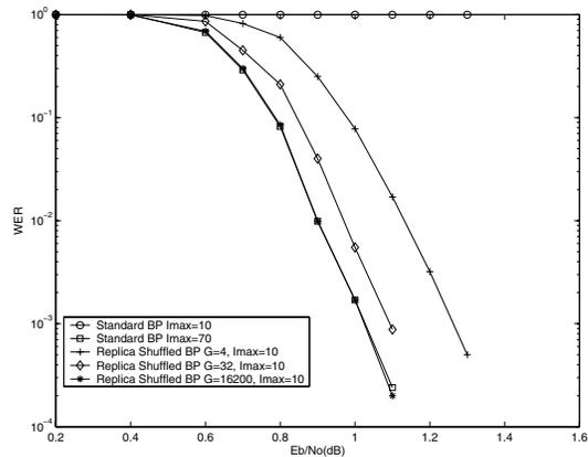
Fig. 6. Error performance for iterative decoding of a (16200, 7200) irregular LDPC code.
