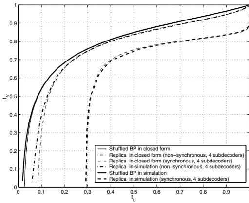
Fig. 3. The comparison between the EXIT functions obtained from the method in [9] and closed form for the (3,6) regular LDPC code at SNR 1.5dB.
