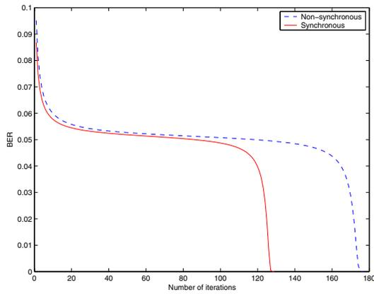
Fig. 2. BER versus number of iterations predicted by density evolution with replica shuffled BP with two subdecoders under non-synchronous and synchronous exchanging schemes, for decoding (3,6) regular LDPC code.
