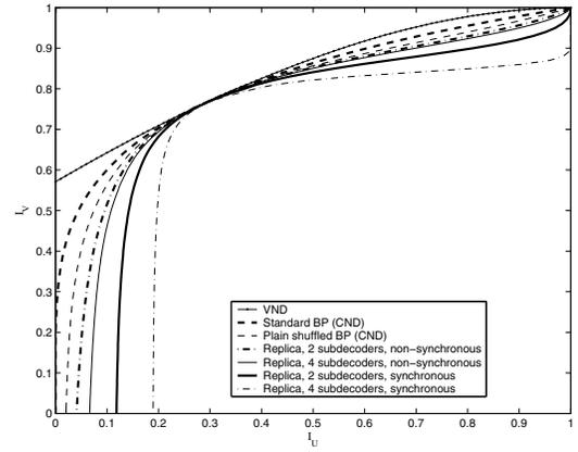
Fig. 5. EXIT curves (in closed form) for standard BP, shuffled BP and four types of replica shuffled BP at 1.11dB.
