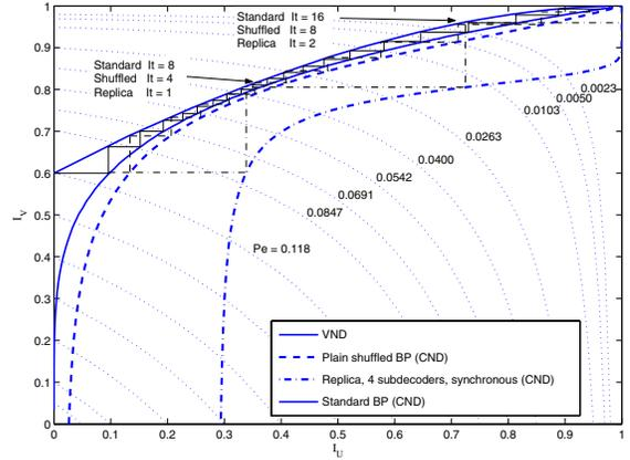
Fig. 4. EXIT curves (in closed form) for standard BP, shuffled BP and replica shuffled BP with four subdecoders and synchronous exchanging scheme at SNR 1.5dB, superimposed to constant-BER curves.
