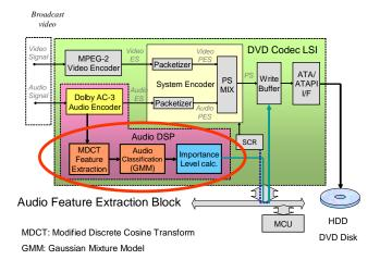
Fig. 1. Simplified Block Diagram for the Recording Phase
