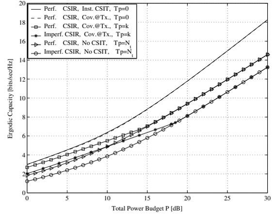
Fig. 6: Ergodic capacity comparison of systems with different CSIT and CSIR assumptions for  $N_t = 2$  and  $N_r = 4$ . ( $T = 10$ ,  $\sigma_\theta = 10^\circ$ ).
