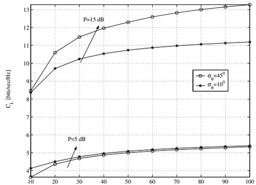
Fig. 1: The impact of the block fading length,  $T$ , on  $C_L$  for  $P = 5$  dB and 15 dB ( $N_t = N_r = 4$ ,  $d_t = 0.5$ ).
