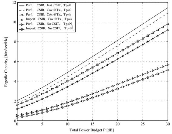
Fig. 7: Ergodic capacity comparison of systems with different CSIT and CSIR assumptions for  $N_t = 4$  and  $N_r = 1$ . ( $T = 10$ ,  $\sigma_\theta = 10^\circ$ ).
