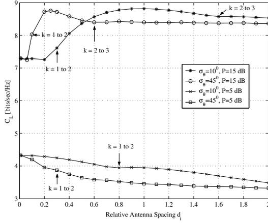
Fig. 3: Impact of the relative antenna spacing,  $d_t$ , on  $C_L$  for  $T = 10$  ( $N_t = N_r = 4$ ,  $P = 15$  dB and 5 dB).
