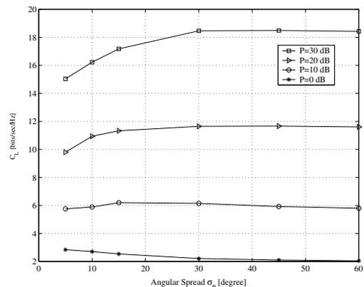
Fig. 2: Impact of the angular spread,  $\sigma_\theta$ , on  $C_L$  ( $N_t = N_r = 4$ ,  $d_t = 0.5$ ,  $T = 10$ ).
