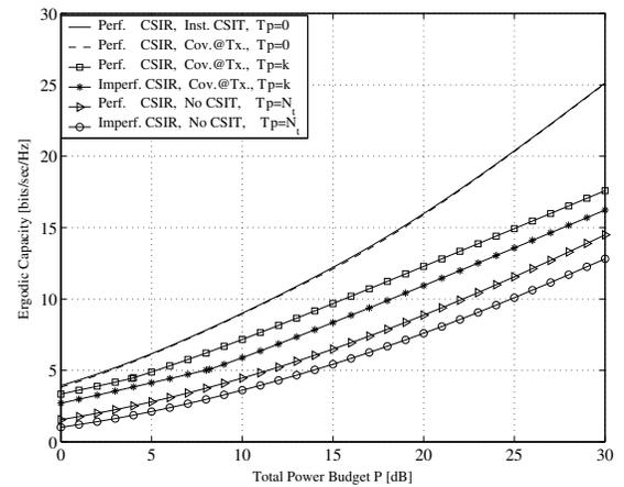
Fig. 8: Ergodic capacity comparison of systems with different CSIT and CSIR assumptions for  $N_t = 4$  and  $N_r = 4$ . ( $T = 10$ ,  $\sigma_\theta = 10^\circ$ ) [11].
