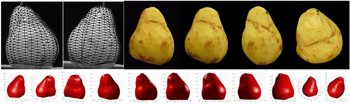
Figure 4: Reconstruction of a pear from 15 views. Left: The mesh superimposed on some original images. Bottom: 3D views of the mesh, with the camera rotating around and then elevating for a view from above. Right: Synthetic views of the pear from viewpoints not spanned by the original camera centers. (Again, the camera orbits and then elevates.) The bottom of the pear is clipped because the occluding contours are incomplete.
