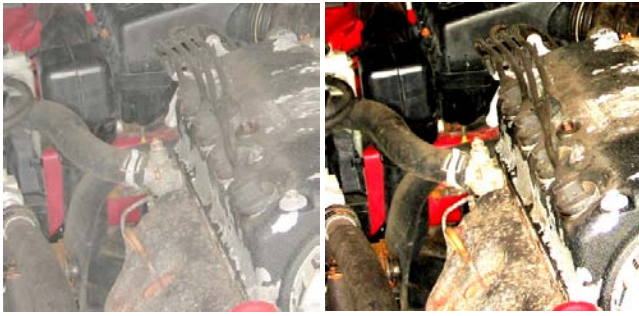
Figure 2: Traditional image enhancement by improving (Left) brightness and (Right) contrast. Low contrast depth edges remain difficult to perceive.
