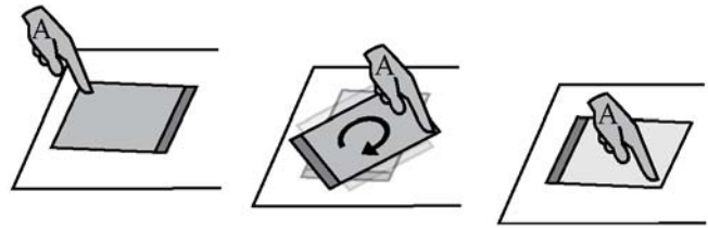
Figure 3. The “reorient” technique for sharing: When User A’s document faces him it is not accessible to other users. User A rotates his document to face the center of the table in order to make it publicly accessible.
