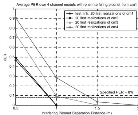
Figure 6 Packet error rate as a function of the distance of interfering piconet in CM 1.
