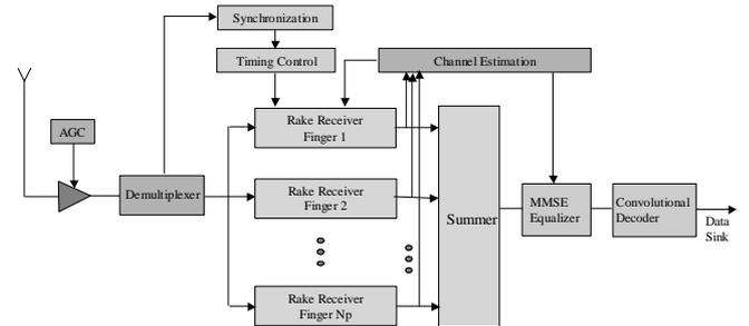
Figure 2 Block diagram of the receiver
