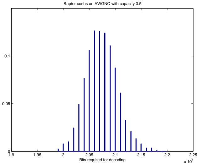
Figure 6: Histogram of number of bits required for successful decoding of raptor code with  $k = 9500$  on an AWGNC with  $E_s/N_0 = -2.83dB$ . The capacity of this channel is 0.5. The receiver first attempts decoding after receiving 19000 noisy bits (Shannon limit). Whenever decoding fails, the receiver waits for another 100 bits before attempting to decode again.
