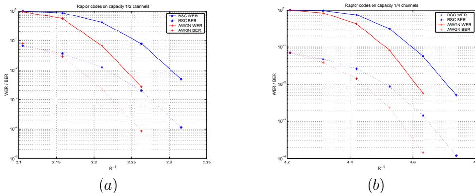
Figure 5: Performance of raptor code with  $k=9500$  and  $k'=10000$  on different channels: (a) BSC with  $p = 0.11$  and AWGNC with  $E_s/N_0 = -2.83dB$ . Both channels have capacity 0.5. (b) on BSC with  $p = 0.2145$  and AWGNC with  $E_s/N_0 = -6.81dB$ . Both channels have capacity 0.25
