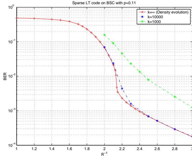
Figure 3: LT codes generated using right distribution in Eqn. 4 on a BSC with  $p = 0.11$
