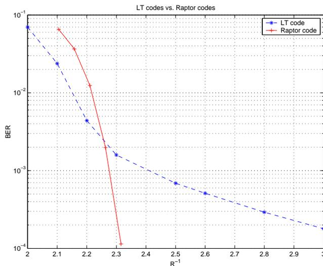
Figure 4: Comparing LT codes with raptor codes on a BSC with  $p=0.11$ . The LT code has  $k = 10000$  and is generated using the distribution in Eqn. 4. The raptor code has  $k = 9500$  and has two components: an outer rate-0.95 LDPC code and an inner rateless LT code generated using the distribution in Eqn. 4.
