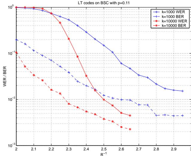
Figure 2: LT codes generated using the  $RS(k,0.01,0.5)$  distribution on a BSC with  $p = 0.11$
