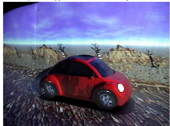
Figure 5: Shearing of the background during acceleration.
