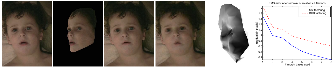
Figure 6: Original frame and three synthetic frames rotating the face, closing the mouth, and pursing the lips. At right is the base shape obtained by feeding the correspondences into the BHB factorization, which inverts the jaw. The graph shows that the flexible factorization estimates morph bases that more effectively explain the data.
