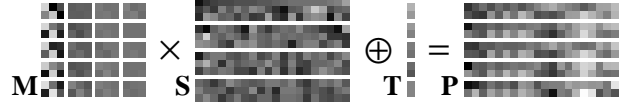
Figure 2: The forward model for multiple frames (eqn. (2)), showing the structure of the motion matrix \mathbf{M} (eqn. (3)). Each block in \mathbf{M} is a scaled rotation matrix; its rows have equal norm and are orthogonal. Moreover, its first row is orthogonal to any second row taken from blocks to the left and right. An SVD of \mathbf{P} \ominus \mathbf{T} produces a pseudo-motion matrix \tilde{\mathbf{M}} = \mathbf{M} \mathbf{J} and pseudo-shape matrix \tilde{\mathbf{S}} = \mathbf{J}^{-1} \mathbf{S} , where \mathbf{J} is an arbitrary unknown full-rank matrix. Successful factorization thus depends on finding a correction matrix \mathbf{J} that will restore the appropriate structure to \tilde{\mathbf{M}} and \tilde{\mathbf{S}} .
