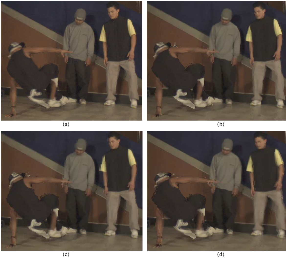
Fig. 7. Comparison of view interpolation quality with QP=27 for texture and various depth encodings. (a) synthesized frame with uncompressed texture and depth, (b) synthesized frame with QP=22 for depth and no sub-sampling, (c) synthesized frame with QP=37 for depth and no sub-sampling, (d) synthesized frame with QP=22 for depth and 4x4 sub-sampling.
