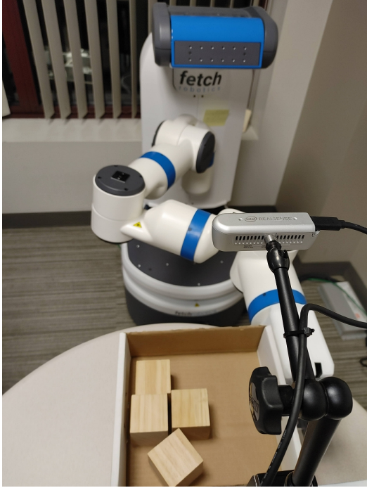
Figure 11. Robotic data collection system used to acquire real-world depth images.
